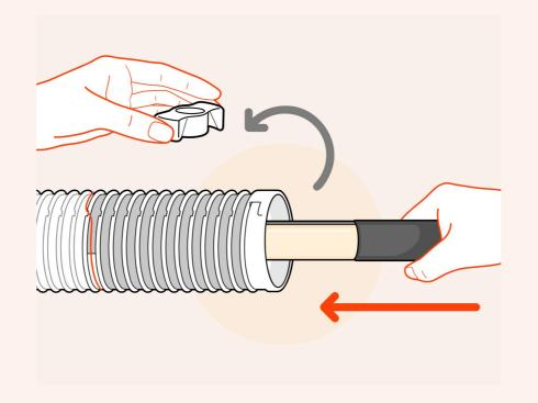
If second exposure is needed, remove the small inner clip to allow the light bar to fit inside the reel to expose the inner reel.
