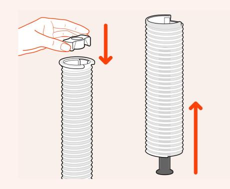
Put the reel together as shown so it's easier to load the film in the dark later.
