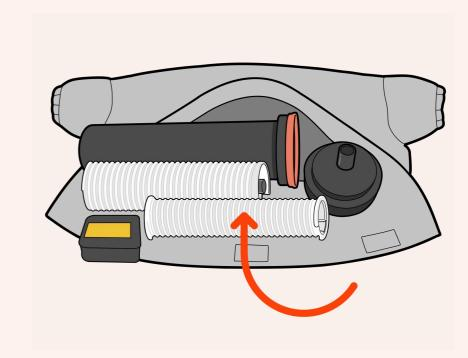
Take reel, film, tank, funnel, roller base and rubber band into the changing bag in preparation for loading film in the dark.
