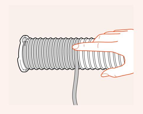
Load the film onto the inner reel, use your finger to guide it into the correct groove.
