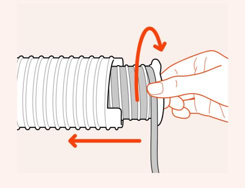
Insert the inner reel into the outer reel and lock them together by twisting inner reel clockwise. The same time hold film in place with your thumb.
